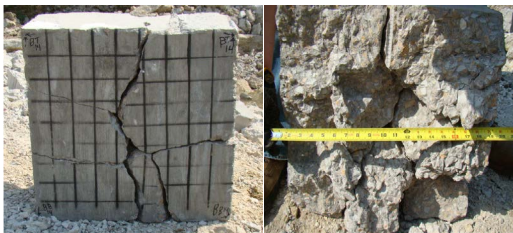
Figure 4.19: Block 14, back face and interior views after impact
