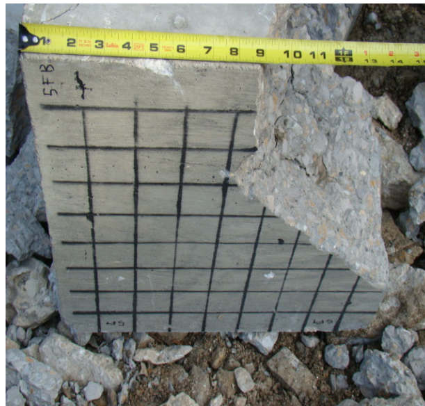
Figure 4.8: Block 5, front face after impact.
