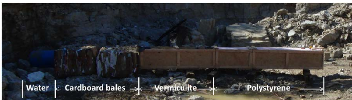
Figure 3.5: Soft recovery system.
