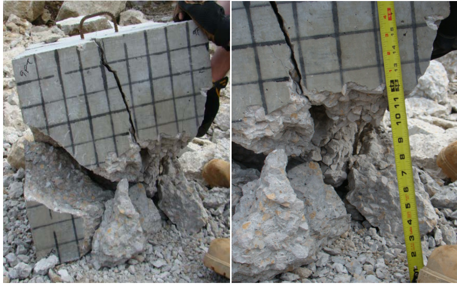
Figure 4.14: Block 9, front face after impact.
